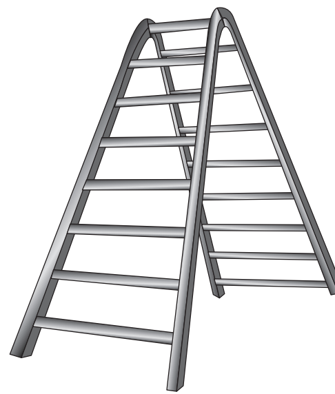
Figure 3.22 A ladder trestle with a height of 4.8 m
