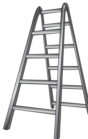
Figure 3.19 A ladder trestle with a height of 3 m
