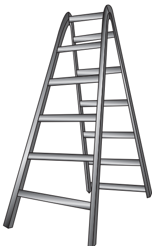
Figure 3.20 A ladder trestle with a height of 3.6 m
