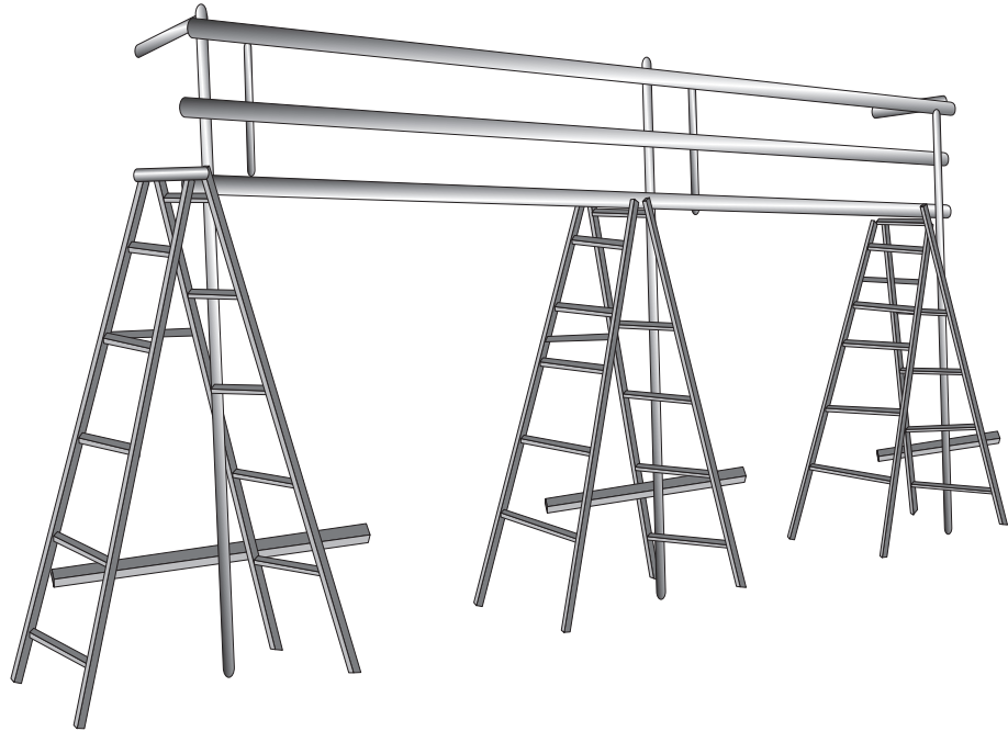
Figure 3.23 Trestles with handrails
