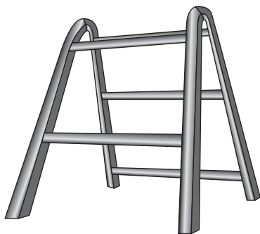
Figure 3.16 A ladder trestle with a height of 1.2 m
