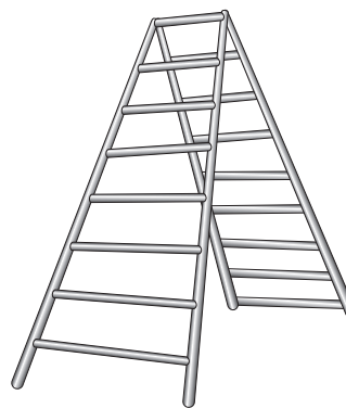
Figure 3.17 A ladder trestle with a height of 1.8 m
